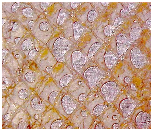
Figure 3. The surface of an adhesive bond which has failed by cohesion due to micro-voiding. The mesh pattern shown is the carrier cloth which has a pitch of 0.5mm (0.020 in.)
